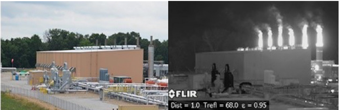
Compressor station emissions made visible with a thermal imaging infrared (FLIR) camera. Photo courtesy of Earthworks.
