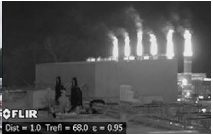
Compressor station emissions made visible with a thermal imaging infrared (FLIR) camera. Photo courtesy of Earthworks.
