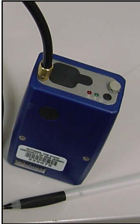
Personal black carbon monitor: 24-hr continuous 1-min. ave. with GPS location
