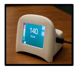
• The Speck, developed by the Carnegie-Mellon University CREATE Lab, is a low-cost, indoor fine particulate (PM<sub>2.5</sub>) monitor. This unit costs \$200.00 and can be purchased at <a href="http://store.specksensor.com/products/speck">http://store.specksensor.com/products/speck</a>.
