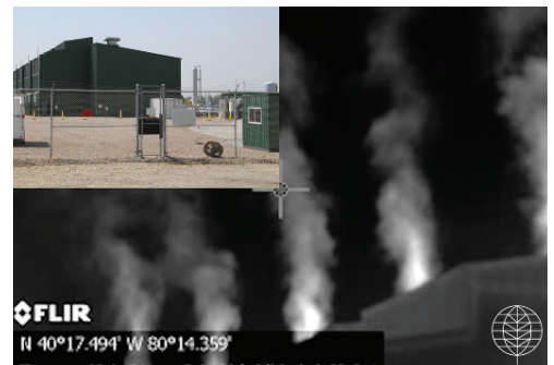
Earthworks' optical gas imaging footage shows normally invisible air pollution at a typical compressor station in southwestern PA
